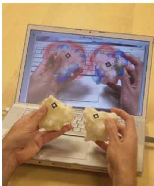
Figure 3.4: Computer augmentation of two subunits of the superoxide dismutase (SOD) dimer, which are tracked and manipulated independently. The electrostatic field is shown with small arrows that point along the local field vectors (they appear as small dots in this picture), and the potential is shown with volume rendered clouds, with positive in blue and negative in red.
